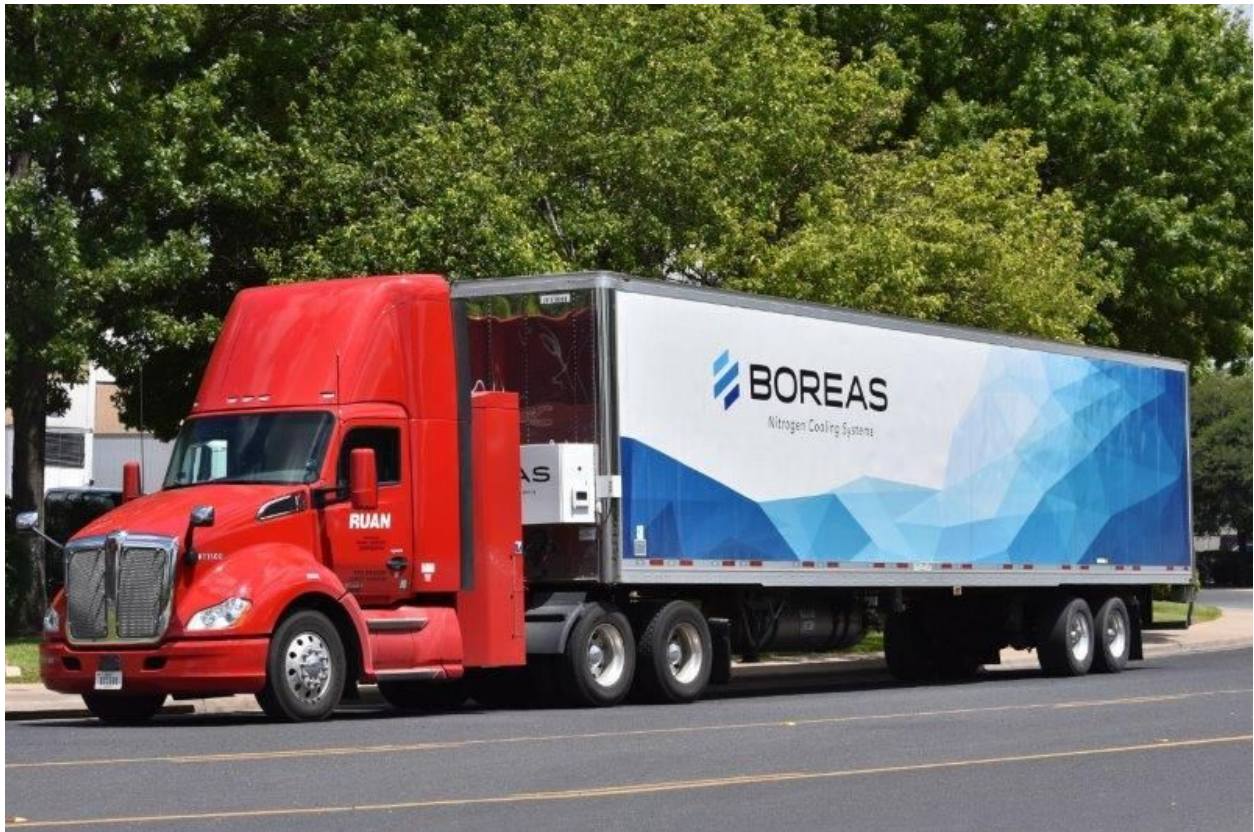
Photo of Ruan RED CNG Tractor and the Boreas Nitrogen Cooling Trailer
